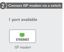
For each ISP modem that has only I port, follow Option 2 in Step 5 when connecting ISP modems to the Bigleaf router. This requires using a simple switch as an indirect connection to the Bigleaf router.
